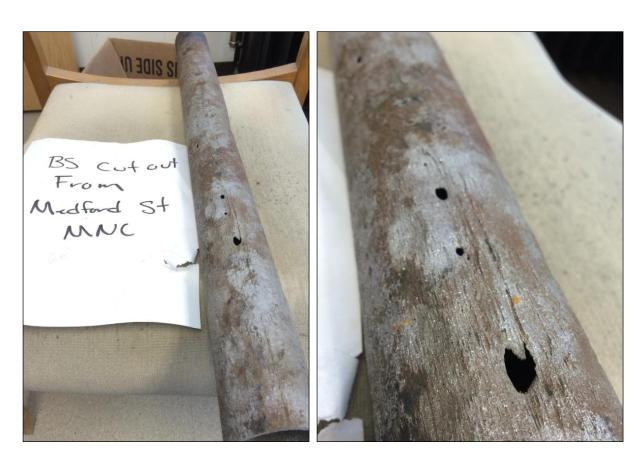
(7) <u>348 Lincoln St (Alley) – WO# 8840-0001000443</u> – 3 inch bare steel (1954), 60 psig pressure – 0.234" wall thickness.
